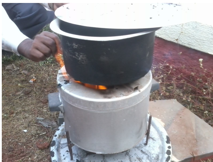
Plate: 5. Water boiling test on cook stove
