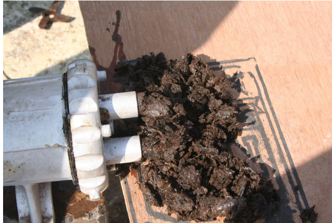
Plate: 1. Briquetting of raw hydrolyzed biomass
